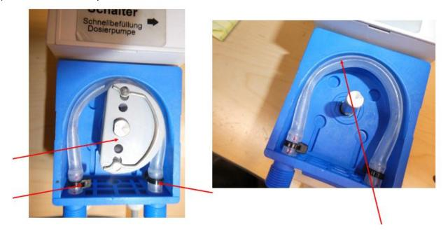
3) Once hose is removed wash and rinse out with white vinegar and massage kink out of affected area, reassemble and return to service.
